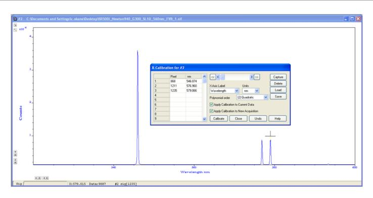
Once the desired number of point have been narrated with the appropriate wavelengths, the 'Manual X-Calibration' can then be applied by selecting the 'Calibrate' button. As you can be observed below, the software applies the required dispersion to the open data.
