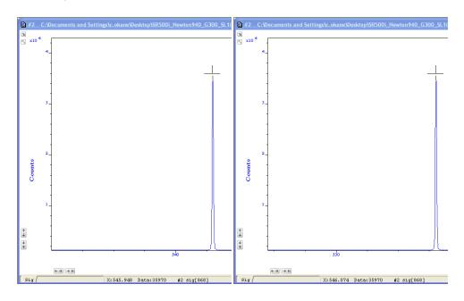
After performing a Manual X-calibration, this can be saved for application to other datasets which are of identical wavelength ranges.
