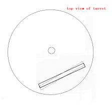
**Roll** This affects how perpendicular the grating grooves are to the system's horizontal axis. The groves should always be vertical; if they are not, different wavelengths will fall at different heights on the sensor. Typically, roll does not need to be adjusted after moving your Shamrock.
