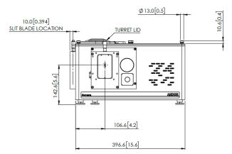
Standard configuration shown with manual slit on input, CCD flange on straight output.
