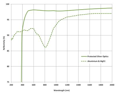
The graph shows the standard Al + MgF<sub>2</sub> optics coatings reflection efficiency versus wavelengths.
