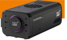
Ultra high speed, low noise, short wave infrared camera, able to run at 600 fps with a readout noise under 30 electrons and a very low dark current <600 e-/p/s.
