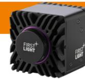
Specially designed for short exposure times applications, C-RED 3 is a very compact high speed VGA uncooled camera for short wave infrared (SWIR) imaging.
